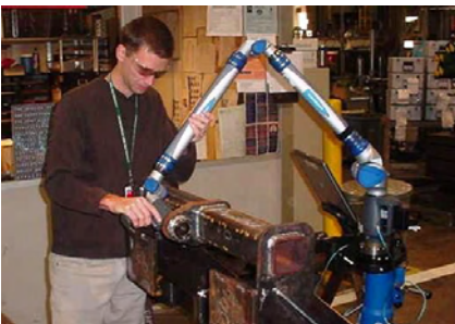
David Wenzel uses the Faro Arm to perform inspection.
